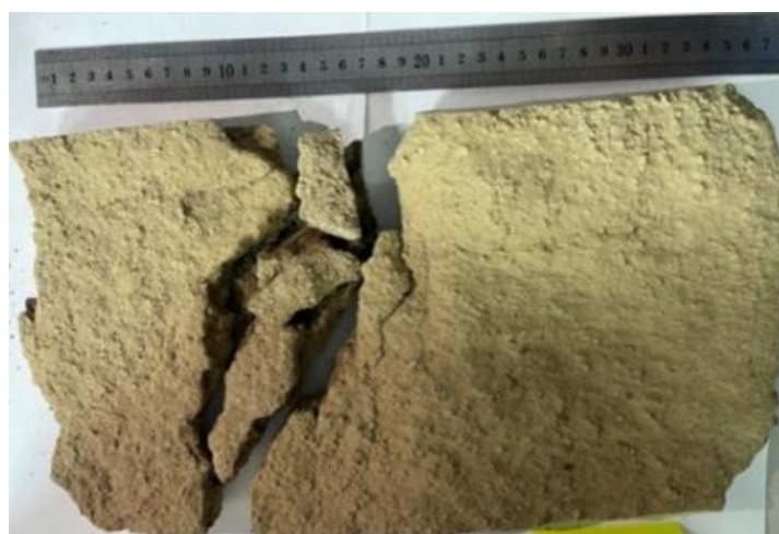
Figure 2 – An example of fixing loam with a two-component resin in the laboratory (author’s material)
